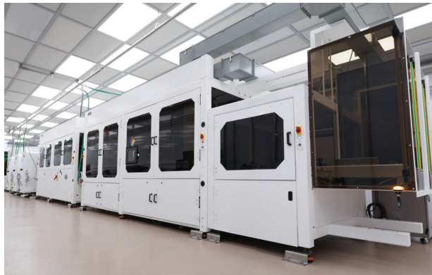
Cell assembly equipment on the Eagle Line
